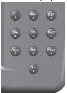
waypoint name. Use data entry keys in conjunction with the **ROCKER**. Press the key once to select the first letter on the key, twice to select the second letter on the key, three times to select the third letter on the key, or four times to select the number on the key. For keys 7, 8, and 9, press the key five times to select the number on the key. When you have selected the correct letter or number, pause, and the unit advances the cursor to the next character automatically.
